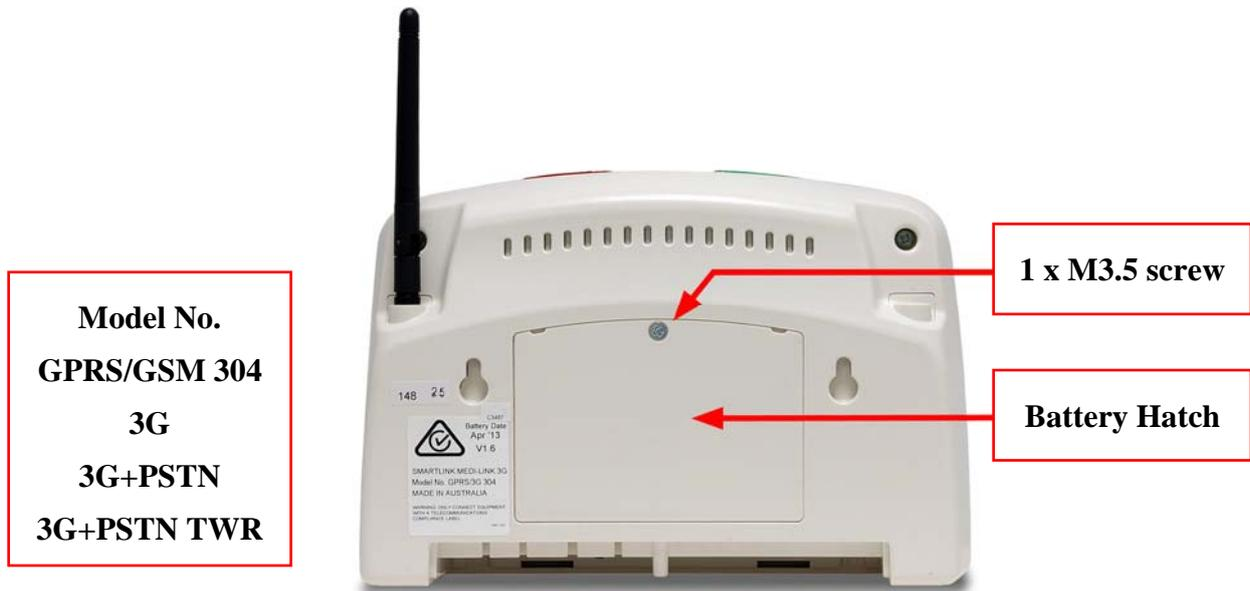
The SIM socket is located beside the battery so remove the Battery first. The SIM socket is a push-push type which is very easy to use. The SIM card needs to be placed contact-side down with the notched corner toward the socket (shown in the diagram below) then pushed in until it clicks into place. When correctly inserted, the edge of the SIM card will not extend into the battery compartment. Upon a second push the SIM card will click out of the SIM socket ready for removal.
